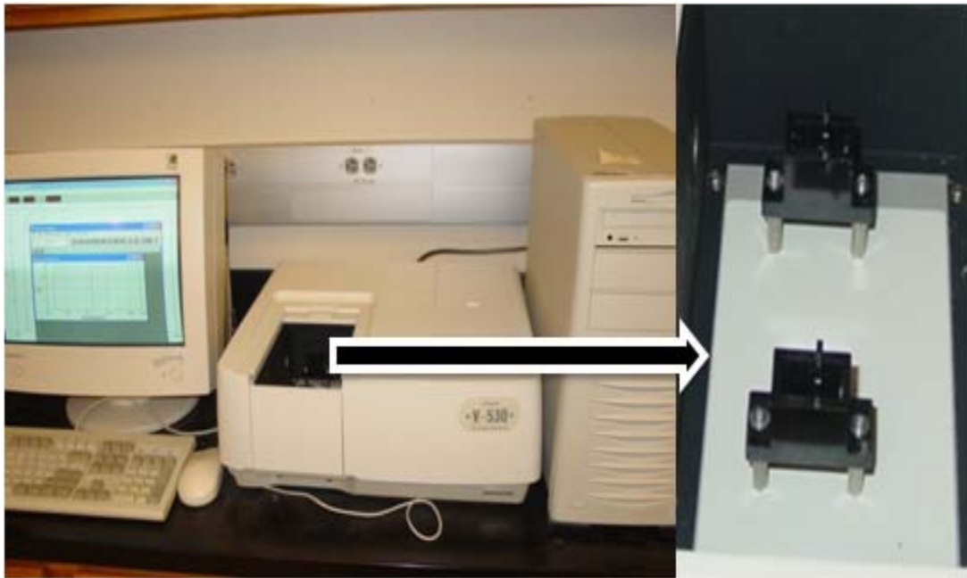
Figure 2.10 UV/vis spectrophotometer with optical system open
