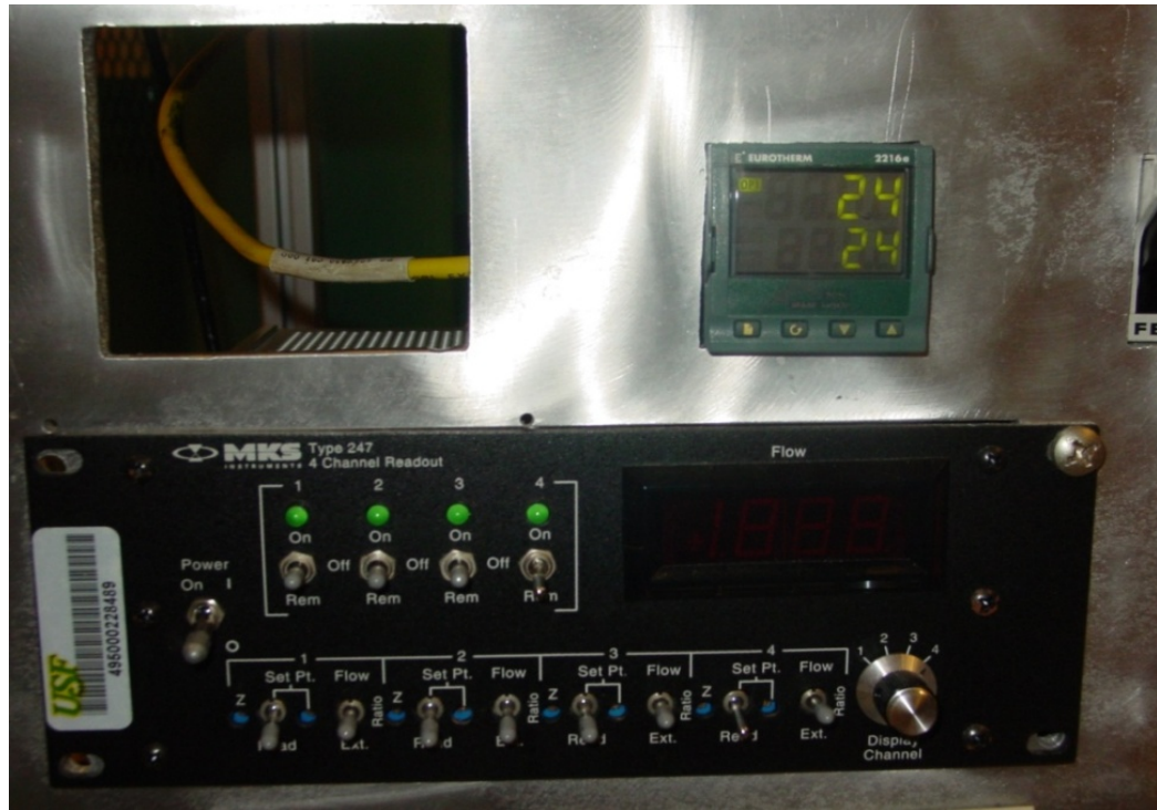
Figure 2.6 Temperature displayed inside the vacuum chamber
